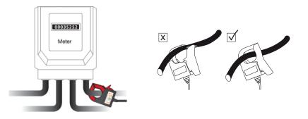
**IMPORTANT:** When looking at the cables leaving the bottom of the meter, they should be fully insulated and you should not be able to see any of the cable conductor or core. **If you do see the live conductor, do not touch the cable and consult a qualified electrical installer for advice.**
